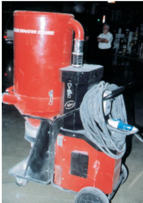
“Up to 98% of the potential airborne grid particles are captured in a vacuum filter during installation of a mechanically installed Polished Concrete Floor System. This allows warehouse workers and valuable stock or cargo items to remain on site during installation.”
