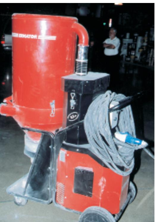
"Up to 98% of the potential airborne grit particles are captured in a vacuum filter during installation of a mechanically installed Polished Concrete Floor System. This allows warehouse workers and valuable stock or cargo items to remain on site during installation."
